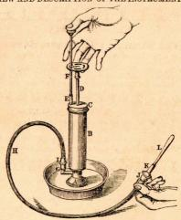
A, Base, connected by a screw, and resting in a basin or vessel. It contains a cavity and valve, through which the fluid in the vessel is drawn into the barrel. B. Barrel. C, Cap. D, Piston. F, Piston standard, inserted into the socket E. G. Elbow. H, Flexible Tube. I, Short metallic coupling. J, Terminal metallic coupling, containing a cavity and valve. K, L, Terminal or injecting tabe, connected with J by a screw.
